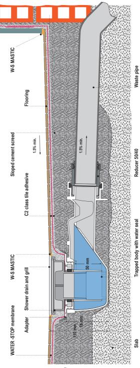
AIKITPLUS eVO installation example with 4 mm flooring thickness
